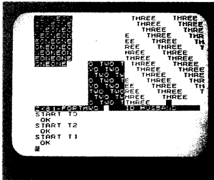
Three tasks are executing, printing the words "one", "two" and "three" at 1, 2 and 3 second intervals. Meanwhile, the keyboard is still available.
